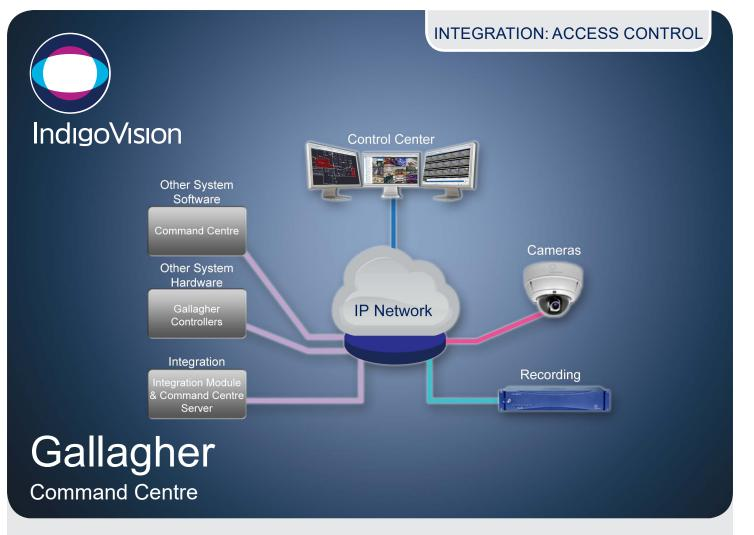
The IndigoVision Gallagher Integration Module allows seamless two-way communication of alarms and events between the Gallagher Command Centre System (formerly Cardax) and IndigoVision's Control Center suite.
