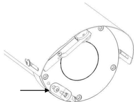
Figure 2 Washer nozzle installation
