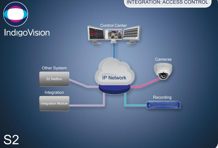
The IndigoVision S2 Integration Module allows alarms and events from the S2 Netbox system to be seamlessly combined with IndigoVision's video security solution, giving complete video and alarm management in a single user interface - Control Center.
