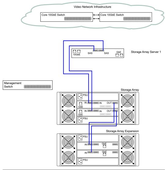
Figure 6: NVR-AS 4000 Large Enterprise System 1000TB - 600 streams - 3000Mbps variant - SAS connections
