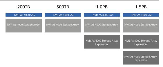
Figure 1: NVR-AS 4000 Large Enterprise System variant components
