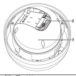
Figure 3 Micro SD card slot
