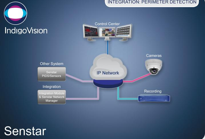
The IndigoVision Senstar Integration Module allows alarms and events from Senstar systems to be seamlessly combined with IndigoVision's video security solution, giving complete video and alarm management in a single user interface - Control Center.
