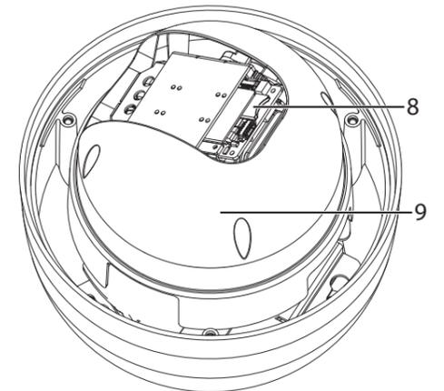
**Figure 3** Micro SD card slot
