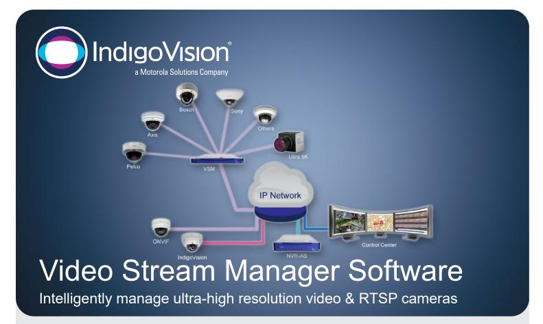
The IndigoVision Video Stream Manager (VSM) enables cameras from a range of other manufacturers to be connected to the IndigoVision Control Center suite by using the industry standard RTSP protocol.
