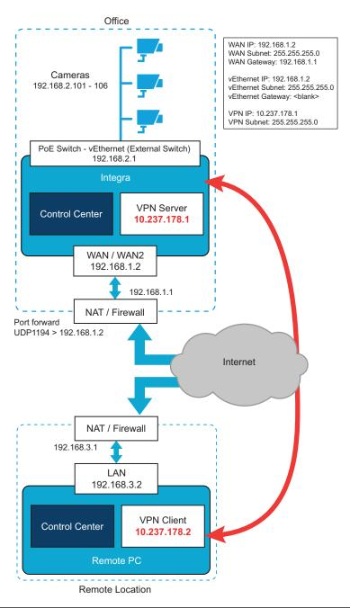
Figure 1: Single Integra with remote access
