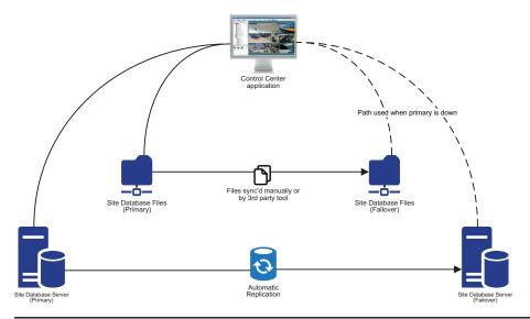
Figure 3: Network configuration with the failover Site Database Server
