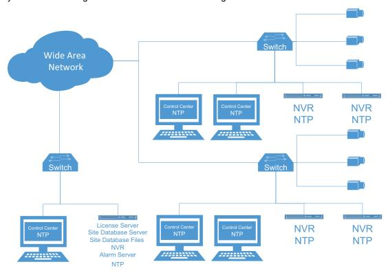
Figure 2: Recommended multiple site architecture
