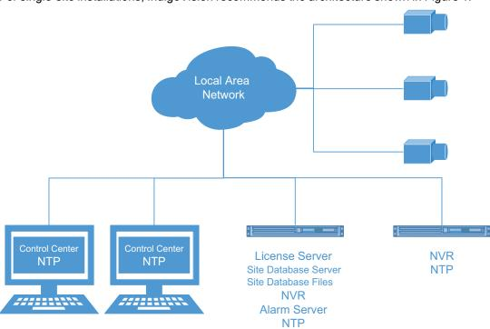
Figure 1: Recommended single site architecture
