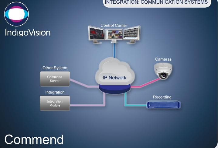
The IndigoVision Commend Integration Module allows events from the Commend intercom system to be seamlessly combined with IndigoVision's video security solution, giving complete video and alarm management in a single user interface - Control Center
