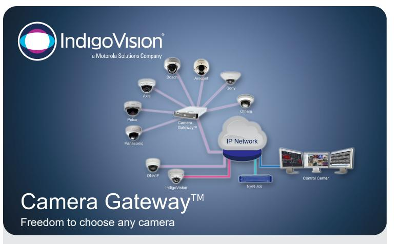
The IndigoVision Camera Gateway<sup>™</sup> enables cameras from a range of other manufacturers to be connected to the IndigoVision Control Center suite. It takes video streams from other manufacturers' cameras using their native protocols and integrates them into the Control Center front-end application.
