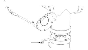
Figure 2 Washer nozzle installation
