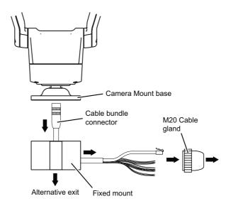
Figure 1 Feed cable bundle through fixed mount and M20 Cable
